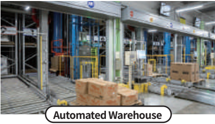
Automated Warehouse This automated warehouse can hold up to 26,500 pallets. Online orders are immediately loaded and unloaded from automated warehouses in order to increase supply efficiency.
